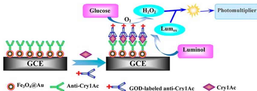
Figure 1. Schematic of the ECL biosensor.
